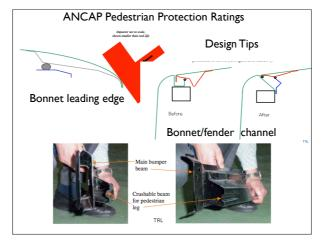
Relatively simple changes to the vehicle can greatly reduce the injury risk to pedestrians. NCAP test labs are working with manufacturers to try and improve designs
