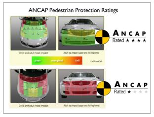
The new Subaru Impreza was the first model to receive a top 4 star pedestrian protection rating from ANCAP. Compare this result with the 1 star rating of the VE Commodore
