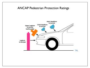
ANCAP commenced pedestrian protection tests at the University of Adelaide in 2000. Four sub-system tests are performed.
