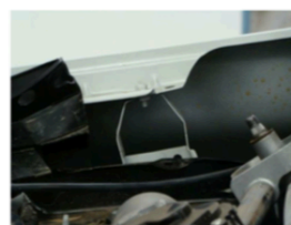
Recent design: Wheel guard supported by collapsible element.
