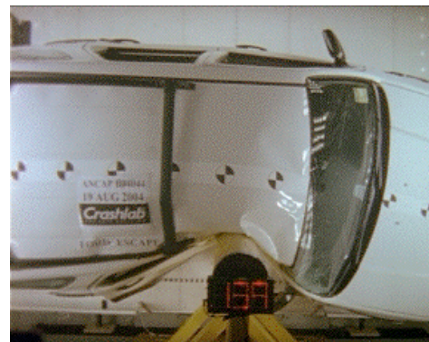
Figure 3. Pole impact test at 29km/h (ANCAP)
