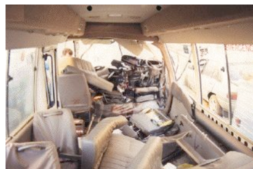
Figure 13. Severe frontal crash of a mid-size bus, showing displaced seats
