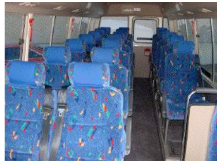
Figure 12. Coaster bus fitted with ADR68 seats
