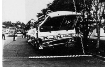
Figure 11a. Roof sway resulting from rollover crash
