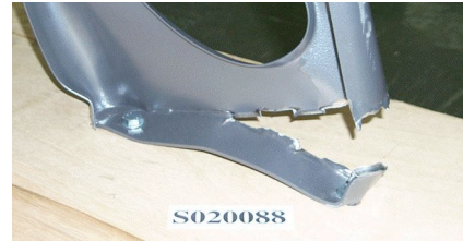
Figure 4a. Pedestal failure during Crashlab sled test (10g)
