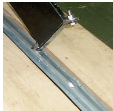
Figure 4b. Floor anchorage failure during Crashlab sled test (10g)
