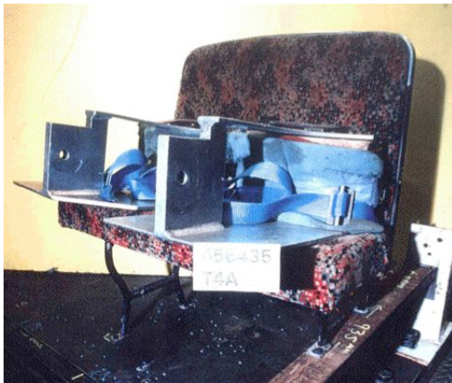
Figure 5. Lap belt test to ECE 14.
