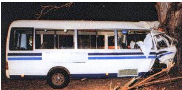
Figure 13. Severe frontal crash of a mid-size bus, showing displaced seats
