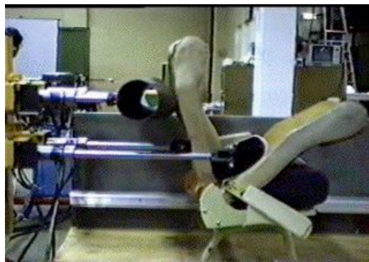
Figure 14b. Crashlab experiment with ECE80 static test procedure
