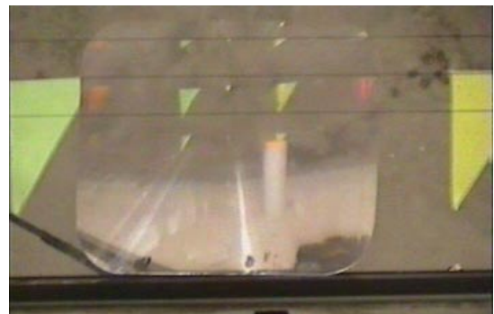
Close up of image in Vanscope. The object at lower right is 2.1m from the vehicle. The cylinder is 4m away.
