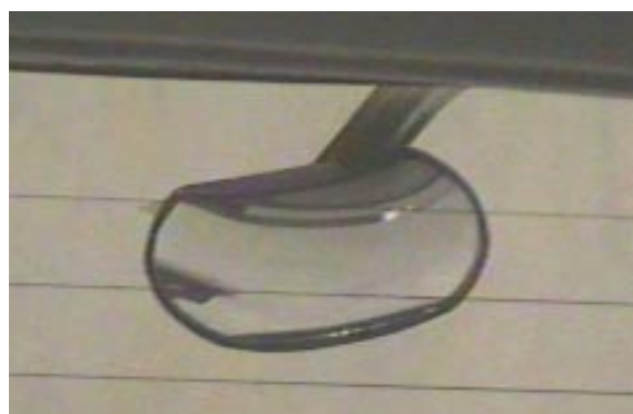
Close up of image in convex mirror. Highly distorted and upside down (the curved object is the bumper bar). The bag is 1m away and the furthest distance (the bottom of the image) is about 1.5m away.
