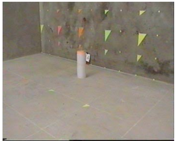
View of factory layout showing the colour-coded grid on the rear wall that was used to measure rearward field of view. Large triangles are 1m apart and high. Small triangles are 0.5 and 1.5m high. The 600mm high test cylinder is also shown.
