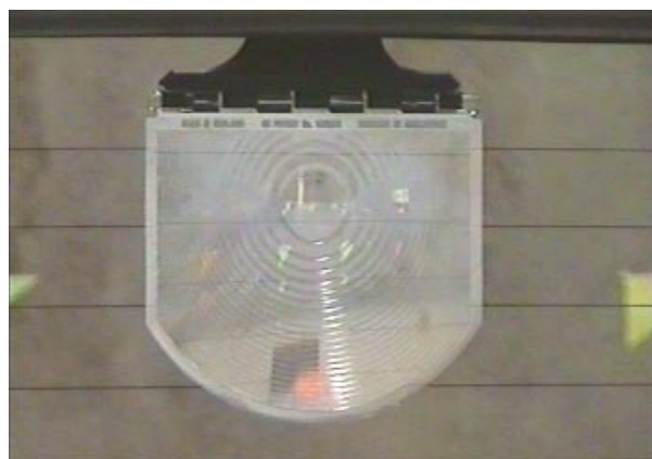
Close up of image in Kwik Park lens. The bag (black object) is 3m from the vehicle. The cylinder (orange top) is 2 m away. The edges of the curved section are 4m away.
