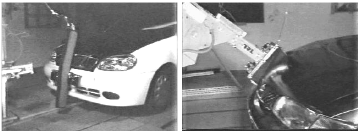
Figure 3a and 3b. Snapshots at peak of Euro NCAP lower and upper legform impact tests (TRL)
