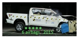
The 64km/h frontal offset test used by most NCAPs has been in use for more than two decades. Regulation R94 is the same but is conducted at 56km/h
