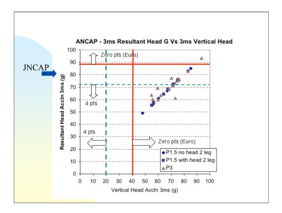
Here are the Australian results for head deceleration. They all perform reasonable well against the proposed Euro NCAP criteria for resultant deceleration (<72g good, >88g poor) but all perform poorly for vertical deceleration (>40g poor). Euro NCAP intends that vertical head deceleration is used as a surrogate for risk of neck injury but there are serious limitations to this assumption, as I will discuss next.
