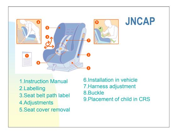
The JNCAP usability tests are illustrated in this picture. They cover instruction manuals, labels, installation of the CRS in the vehicle and securing the child in the CRS.
