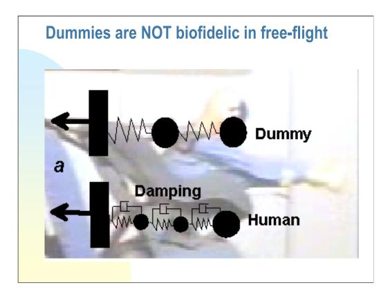
Injury criteria apply to specific models of child dummy. Identical RTA sled tests produced a head deceleration of 200g in a TNO P-Series dummy and 60g in a CRABI dummy. This should alert us a problem with dummy biofidelity in this type of crash simulation.
