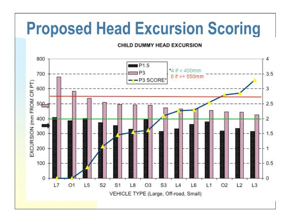
It is considered that a sliding scale is more appropriate than a step function for assessing head excursion. This will reward CRS that perform exceptionally well at limiting head excursion. It will also help to reduce the effects of the uncertainty in measuring head excursion - due mainly to parallax effects.
