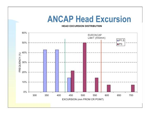
This graph show the distribution of head excursion for 14 ANCAP tests. As expected, the head excursion for the shorter, lighter P1.5 dummy is less than that of the P3 dummy. In two Australian tests the head excursion of the P3 dummy exceeded 550mm.
