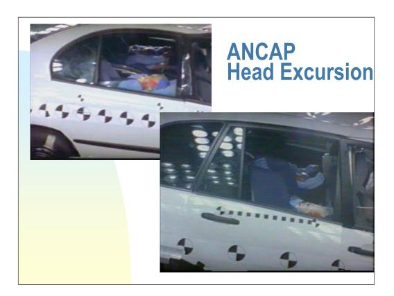
In one case the lower part of the CRS was poorly restrained by the adult seat belt - this is shown in the top picture.
