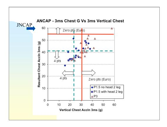
Here are the Australian results for chest deceleration. They perform reasonably well for the resultant chest g (<41g good, >55g poor) but poorly with vertical chest deceleration (>30g poor). My concern is that, although vertical chest deceleration is prescribed in the ECE Regulation, it is only intended to relate to *compression* of the spine that might occur with rearward facing CRS. Limiting *tension* in the spine, as occurs with forward facing CRS, does not make sense.
