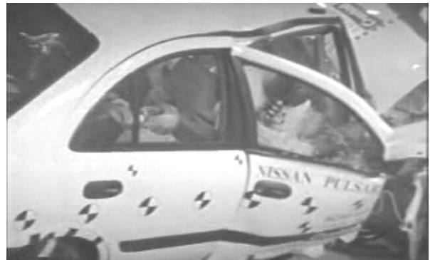
ANCAP Offset Frontal Crash at 64km/h
