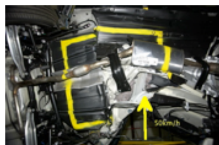
Very severe 50k/h pole test of same model sedan
