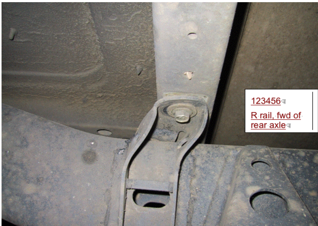
Figure 7: Seat anchorage structure in unitary construction vehicles will typically include both welded and bolted connections. Photograph shows unrepaired accident damage to primary connections which probably makes retrofitting uneconomic.
